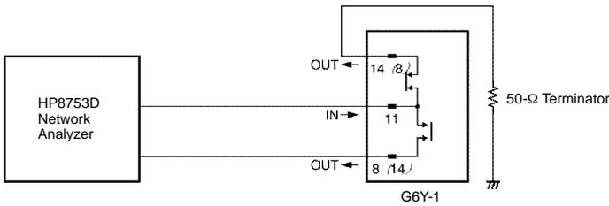
Terminals which were not being measured were terminated with 50  $\Omega$ .
