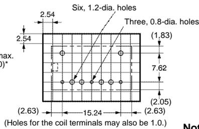
**Terminal Arrangement/ Internal Connections (Bottom View)**
