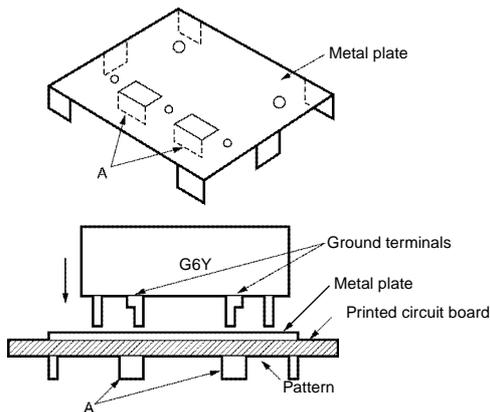
With this method a metal plate is placed between the Relay and base and connected to the pattern, as shown in the above diagram.
