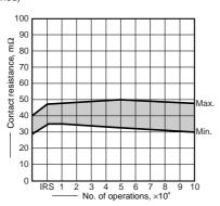
4.-(2) Electrical life (0.5 Å 125 V AC resistive load) Tested sample: TQ2SA-12V, 6 pcs. Operating frequency: 20 cpm Change of pick-up and drop-out voltage (mounting by IRS method)
