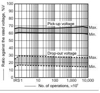
4-.(1) Electrical life (2 Å 30 V DC resistive load) Tested sample: TQ2SA-12V, 6 pcs. Operating frequency: 20 cpm Change of pick-up and drop-out voltage (mounting by IRS method)
