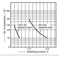
3. Mechanical life (mounting by IRS methad) Tested sample: TQ2SA-12V, 10 pcs.
