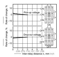
14. Pulse dialing test Tested sample: TQ2SA-12V, 6 pcs. (35 mA 48 V DC wire spring relay load)
