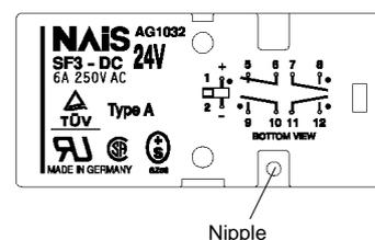
If required a breathing hole can be made in the cover by removing the nipple. However be aware that the degree of protection will reduce from IP67 to IP30!
