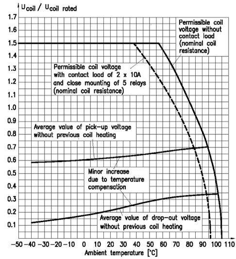
Permissible coil voltages and pick-up and drop-out characteristics at various ambient temperatures.
