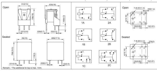
Remark:1) In case of no tolerance shown in outline dimension: outline dimension ≤1mm,tolerance should be ±0.2mm; outline dimension >1mm and ≤5mm,tolerance should be ±0.3mm;outline dimension >5mm, tolerance should be ±0.4mm.
