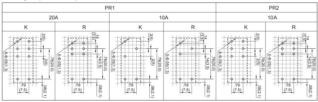
Remark:1) In case of no tolerance shown in outline dimension: outline dimension ≤1mm,tolerance should be ±0.2mm; outline dimension >1mm and ≤5mm,tolerance should be ±0.3mm; outline dimension >5mm, tolerance should be ±0.4mm.
