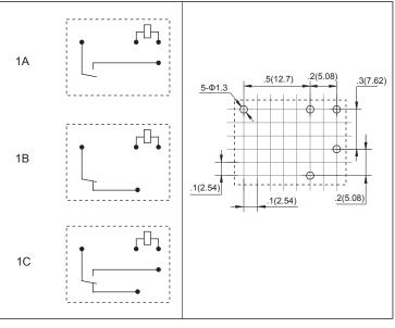
Remark:1) In case of no tolerance shown in outline dimension: outline dimension ≤1mm,tolerance should be ±0.2mm; outline dimension >1mm and ≤5mm,tolerance should be ±0.3mm;outline dimension >5mm, tolerance should be ±0.4mm.
