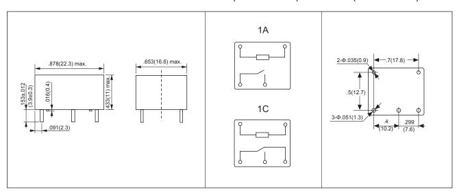
Remark:1) In case of no tolerance shown in outline dimension: outline dimension ≤1mm,tolerance should be ±0.2mm; outline dimension >1mm and ≤5mm,tolerance should be ±0.3mm;outline dimension >5mm, tolerance should be ±0.4mm.
