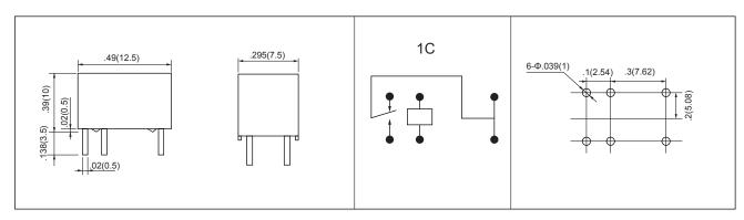
Remark:1) In case of no tolerance shown in outline dimension: outline dimension ≤1mm,tolerance should be ±0.2mm; outline dimension >1mm and ≤5mm,tolerance should be ±0.3mm;outline dimension >5mm, tolerance should be ±0.4mm.
