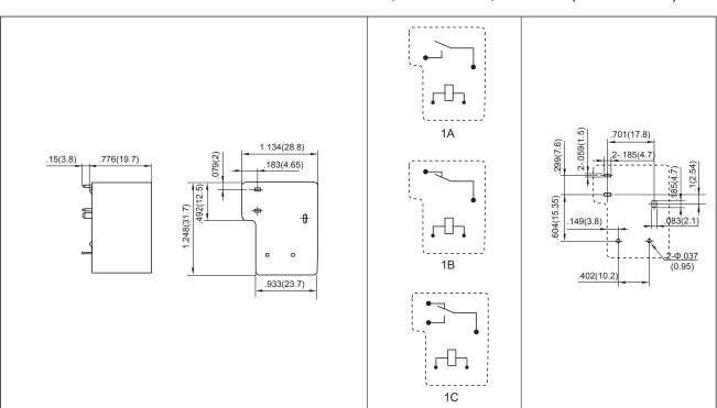
Remark:1) In case of no tolerance shown in outline dimension: outline dimension ≤1mm,tolerance should be ±0.2mm; outline dimension >1mm and ≤5mm,tolerance should be ±0.3mm;outline dimension >5mm, tolerance should be ±0.4mm.
