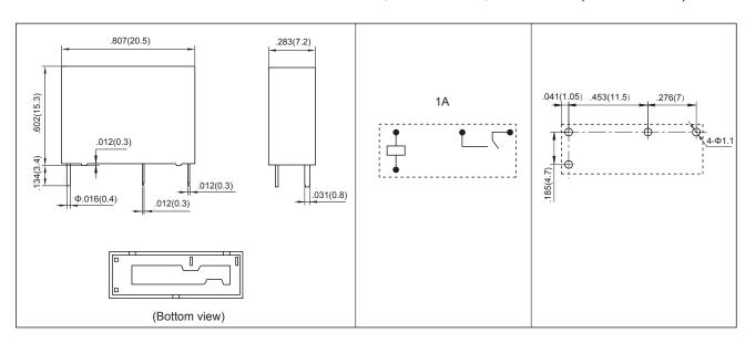
Remark:1) In case of no tolerance shown in outline dimension: outline dimension  $\leq$ 1mm,tolerance should be  $\pm$ 0.2mm; outline dimension >1mm and  $\leq$ 5mm,tolerance should be  $\pm$ 0.3mm;outline dimension >5mm, tolerance should be  $\pm$ 0.4mm.
