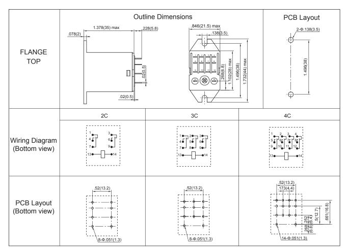
Remark:1) In case of no tolerance shown in outline dimension: outline dimension ≤1mm,tolerance should be ±0.2mm; outline dimension >1mm and ≤5mm,tolerance should be ±0.3mm;outline dimension >5mm, tolerance should be ±0.4mm.
