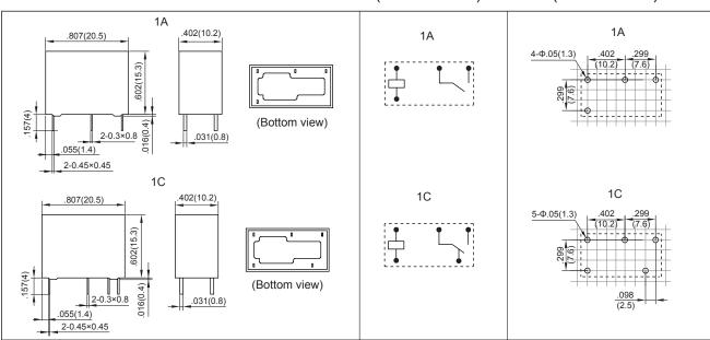
Remark:1) In case of no tolerance shown in outline dimension: outline dimension ≤1mm,tolerance should be ±0.2mm; outline dimension >1mm and ≤5mm,tolerance should be ±0.3mm;outline dimension >5mm, tolerance should be ±0.4mm.
