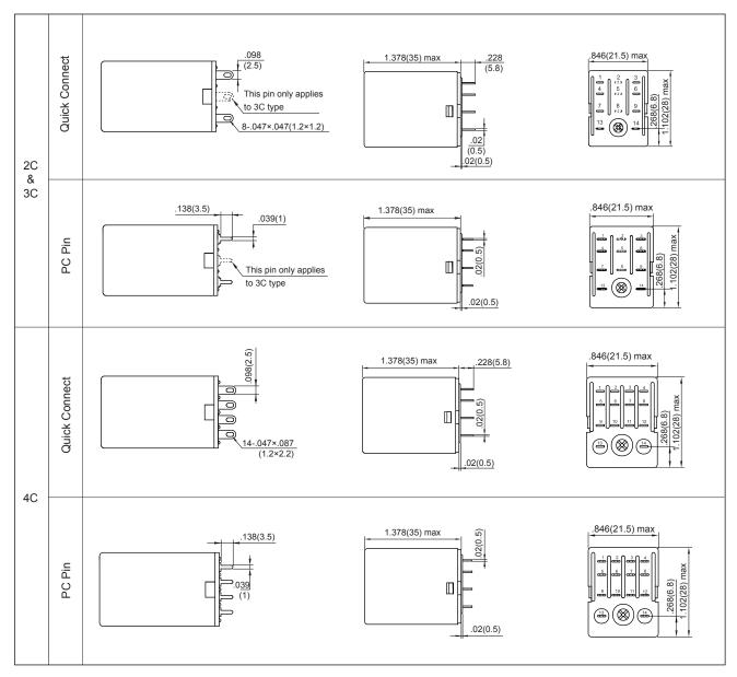
Remark:1) In case of no tolerance shown in outline dimension: outline dimension ≤1mm,tolerance should be ±0.2mm; outline dimension >1mm and ≤5mm,tolerance should be ±0.3mm;outline dimension >5mm, tolerance should be ±0.4mm.
