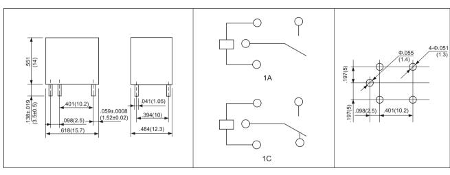
Remark:1) In case of no tolerance shown in outline dimension: outline dimension ≤1mm,tolerance should be ±0.2mm; outline dimension >1mm and ≤5mm,tolerance should be ±0.3mm;outline dimension >5mm, tolerance should be ±0.4mm.
