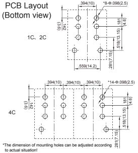
Remark:1) In case of no tolerance shown in outline dimension: outline dimension ≤1mm,tolerance should be ±0.2mm; outline dimension >1mm and ≤5mm,tolerance should be ±0.3mm;outline dimension >5mm, tolerance should be ±0.4mm.
