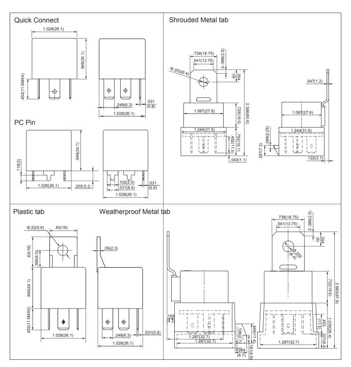
Remark:1) In case of no tolerance shown in outline dimension: outline dimension ≤1mm,tolerance should be ±0.2mm; outline dimension >1mm and ≤5mm,tolerance should be ±0.3mm;outline dimension >5mm, tolerance should be ±0.4mm.
