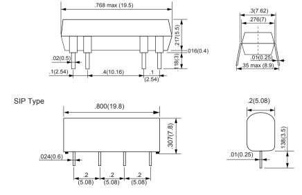
Remark:1) In case of no tolerance shown in outline dimension: outline dimension  $\leq$ 1mm,tolerance should be  $\pm$ 0.2mm; outline dimension  $\geq$ 1mm and  $\leq$ 5mm,tolerance should be  $\pm$ 0.3mm;outline dimension  $\geq$ 5mm, tolerance should be  $\pm$ 0.4mm.
