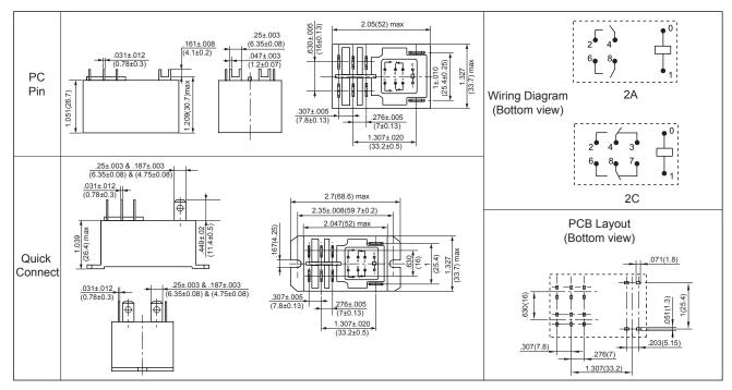
Remark:1) In case of no tolerance shown in outline dimension: outline dimension ≤1mm,tolerance should be ±0.2mm; outline dimension >1mm and ≤5mm,tolerance should be ±0.3mm;outline dimension >5mm, tolerance should be ±0.4mm.
