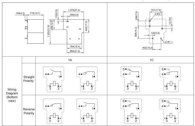
Remark:1) In case of no tolerance shown in outline dimension: outline dimension ≤1mm,tolerance should be ±0.2mm; outline dimension >1mm and ≤5mm,tolerance should be ±0.3mm;outline dimension >5mm, tolerance should be ±0.4mm.
