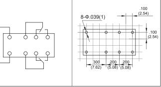
Remark:1) In case of no tolerance shown in outline dimension: outline dimension ≤1mm,tolerance should be ±0.2mm; outline dimension >1mm and ≤5mm,tolerance should be ±0.3mm;outline dimension >5mm, tolerance should be ±0.4mm.
