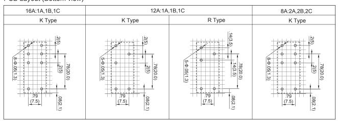
Remark:1) In case of no tolerance shown in outline dimension: outline dimension ≤1mm,tolerance should be ±0.2mm; outline dimension >1mm and ≤5mm,tolerance should be ±0.3mm;outline dimension >5mm, tolerance should be ±0.4mm.
