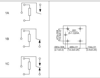
Remark:1) In case of no tolerance shown in outline dimension: outline dimension ≤1mm,tolerance should be ±0.2mm; outline dimension >1mm and ≤5mm,tolerance should be ±0.3mm;outline dimension >5mm, tolerance should be ±0.4mm.
