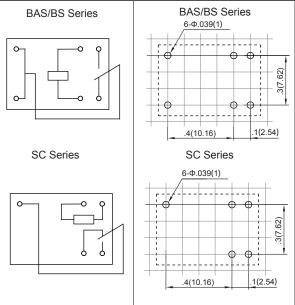
Remark:1) In case of no tolerance shown in outline dimension: outline dimension  $\leq$ 1mm,tolerance should be  $\pm$ 0.2mm; outline dimension  $\geq$ 1mm and  $\leq$ 5mm,tolerance should be  $\pm$ 0.4mm.
