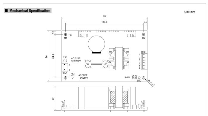
AC Input Connector (CN1): Molex 5277-02 or equivalent
