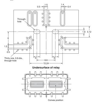
Note: When higher isolation is required, connect the convex position on the undersurface of the relay to the ground pattern of the substrate by soldering
