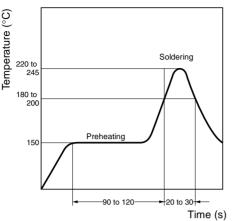
Note: Temperatures indicate the surface temperatures of the PCB
